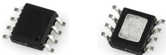
(Fig. 1) An image of a plastic encapsulated SOIC8 package.
