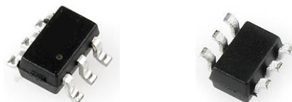
(Fig. 1) An image of a plastic encapsulated SOT363 package.
