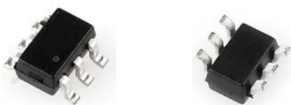
(Fig. 1) An image of a plastic encapsulated SOT363 package.
