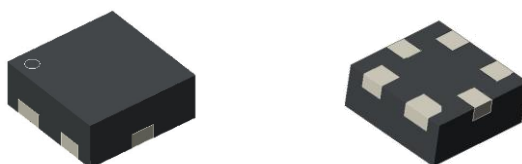
(Fig. 1) An image of a plastic encapsulated UQFN6 package.
